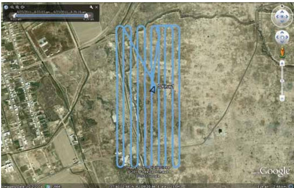
**Fig. 9:** Tracklog of a single flight in the north-west of Sultan Kala (output as a kml file from the software and displayed on the Google Earth satellite image). The UAV took off north-west from near the centre of the survey area, before starting the systematic north-south runs pre-programmed in the flight plan.
