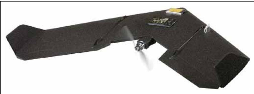
**Fig. 6:** The *swinglet* CAM UAV (© senseFly LLC).
