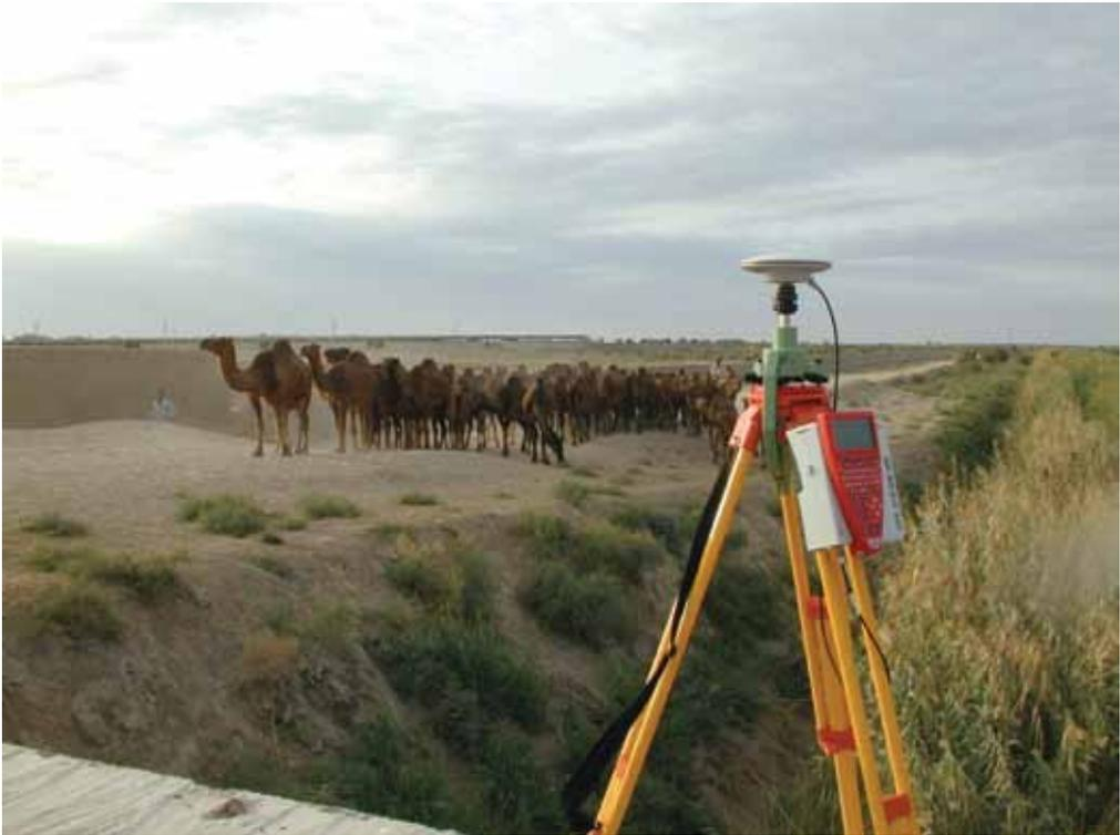
**Fig. 5:** The Leica Global Positioning System (GPS) set up to establish a control point, on one of the road bridges near Ancient Merv, to geo-reference the IKONOS satellite image.
