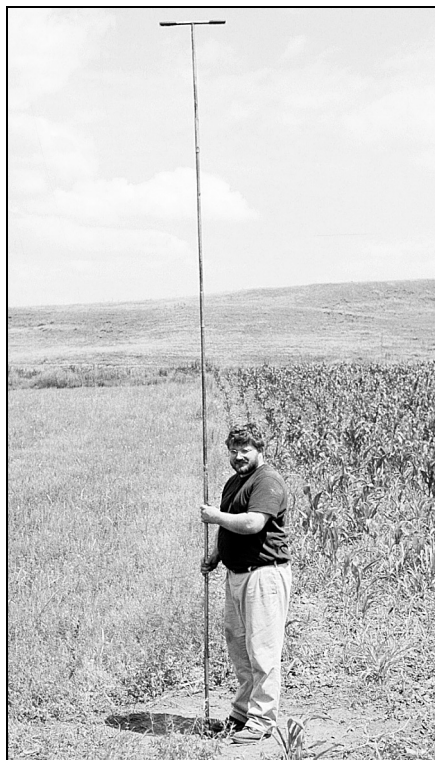
Figure 8 Taking sediment samples in the area of the putative Roman harbour at Noviodunum, using a hand auger down to a depth of 4.5 m (auger hole 1 on Fig. 5).
