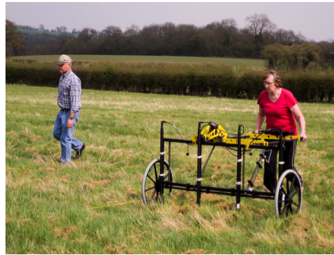
Fig. 2: Magnetometry survey in progress in Hertfordshire as part of the AHRC-funded project 'Sensing the Iron Age and Roman Past' (photo: Kris Lockyear).
