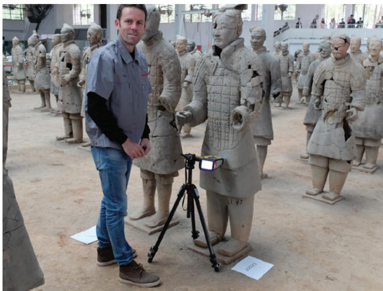
**Figure 1** Patrick Quinn characterising the composition of statues of Emperor Qin Shihuang's Terracotta Army, China, via non-destructive portable X-ray fluorescence spectroscopy. This research detected chemical differences that are indicative of the production of statues by two separate workshops working on the first emperor's mausoleum (Quinn et al. 2020)
