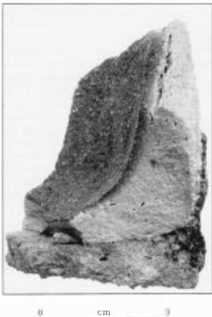
Figure 1 A crucible fragment from Gyaur Kala, Merv, showing a cross section through the lower wall and the supporting pad below.
