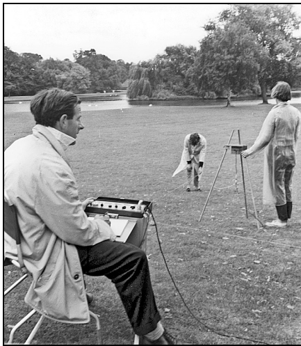
Figure 8 Martin Aitken using his proton magnetometer at Verulamium in 1959 to locate the "1955 Ditch" below the surface.
