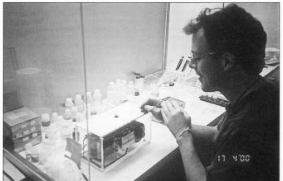
Figure 1 The author loading purified strontium onto a tungsten filament for analysis by thermal-ionization mass spectrometry.
