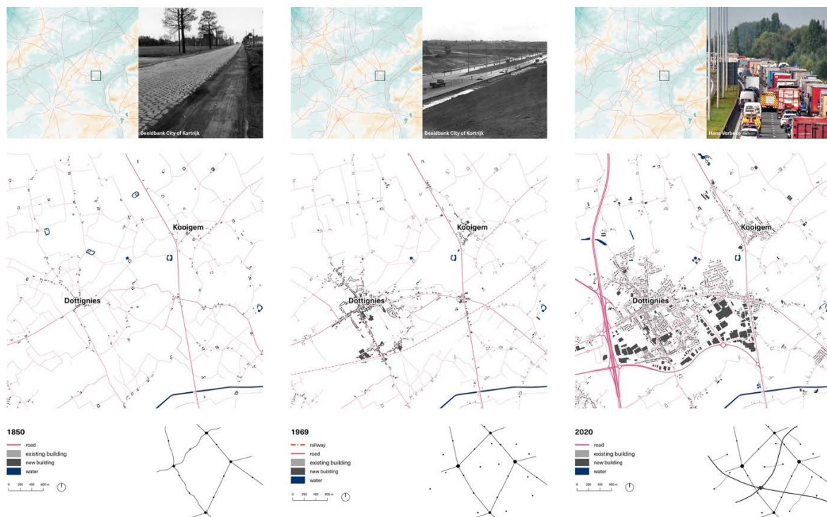
Figure 10. The evolution of the territory around Dottignies (Wallonia) and Kooigem (Flanders) between 1850 and 2020 through the perspective of individual-mobility networks. While initially, paved roads were rare, the introduction of highways and the increased asphaltting of local roads facilitated the development of residential allotments and an industry park with good accessibility (Source: from Sophie Leemans, based on data from Google Earth; OSM; Geopunt Vlaanderen; Géoportail de la Wallonie; NGL/IGN Belgium; IGN France, 2020)
