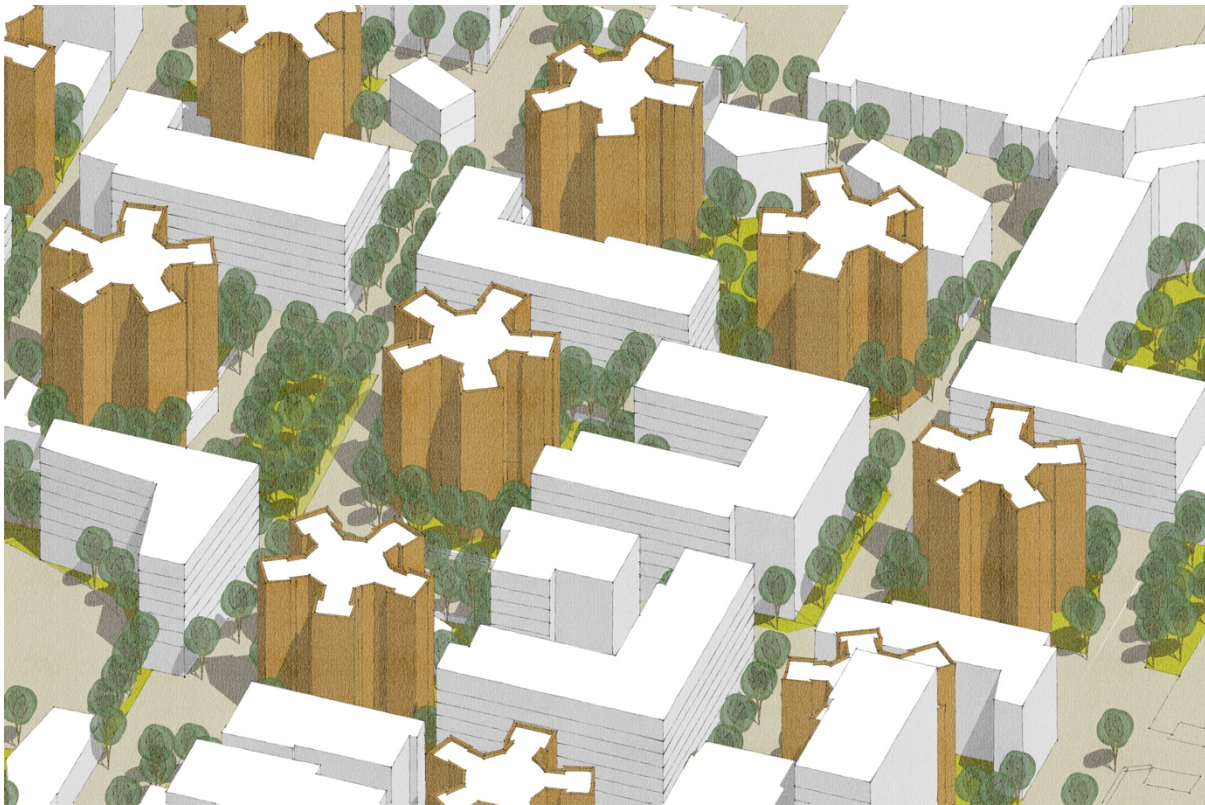
Figure 6. Diagram of infill development forming streets and public squares in coordination with existing towers
