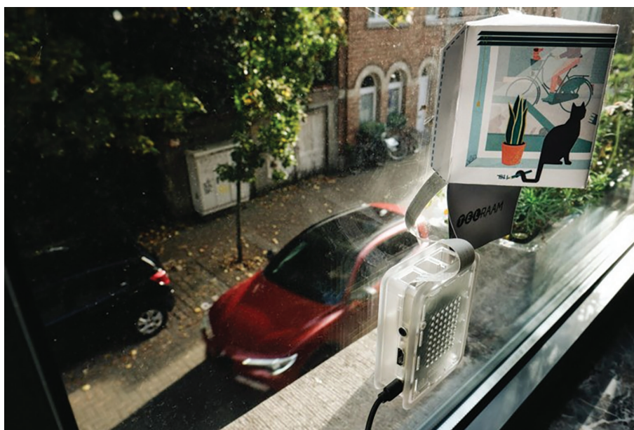
Figure 1. A Telraam traffic sensor attached to a window (Source: WeCount project)
