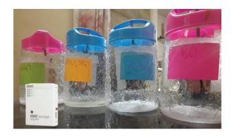
Preliminary trials were carried out by trial and error to fix the amount of salt and water to obtain the specific RH value. The temperature and RH loggers (Hobo U10, Onset, USA) were attached on the inner side of the lid of the jars to ensure constant RH inside the containers.
