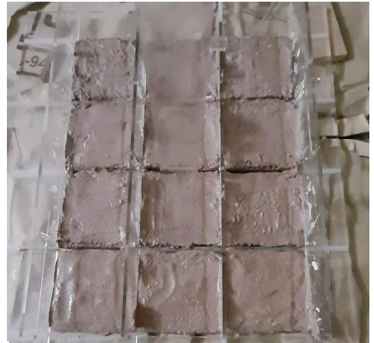
Figure 57 Lime Plaster samples in a battery mold for curing.
