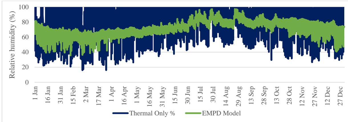
Figure 8 Relative Humidity BESTEST Model of Thermal Only and EMPD.
