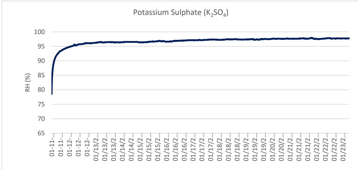
Figure 54 96% RH maintained by K<sub>2</sub>SO<sub>4</sub>
