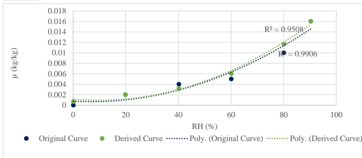
Figure 1 Best fitted sorption curve for lime plaster.
