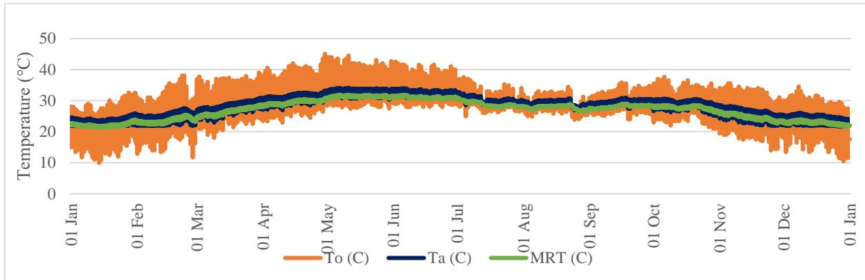
Figure 10 Simulations results showing a range of outdoor, indoor, and mean radiant temperature in PT\_B.
