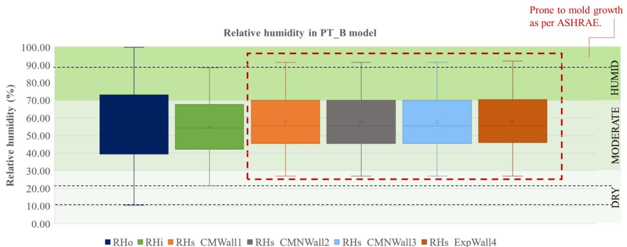
Figure 11 Relative Humidity levels of space and on the surface of the walls in PT\_B.
