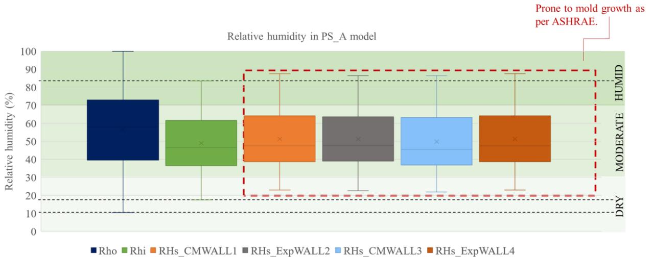
Figure 14 Relative Humidity levels of space and on the surface of the walls in PS\_A.
