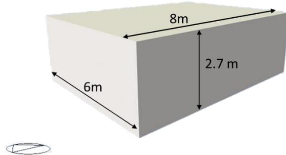
Figure 36 Sorption curve used for simulations. Figure 37 BESTEST Model Used for simulations.
