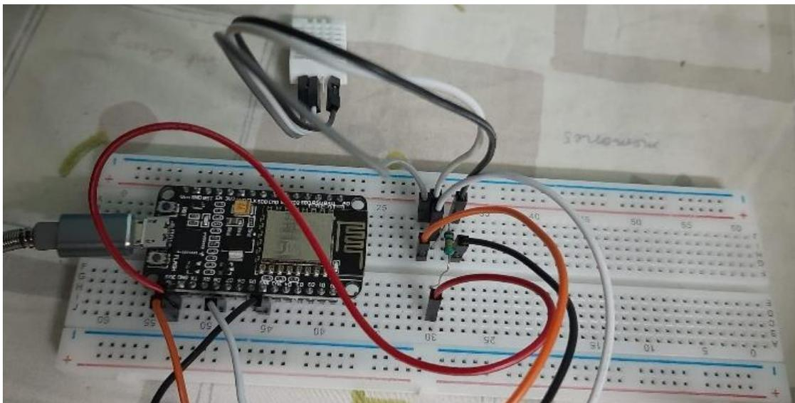
Figure 51 RH sensor circuit for logging RH levels
