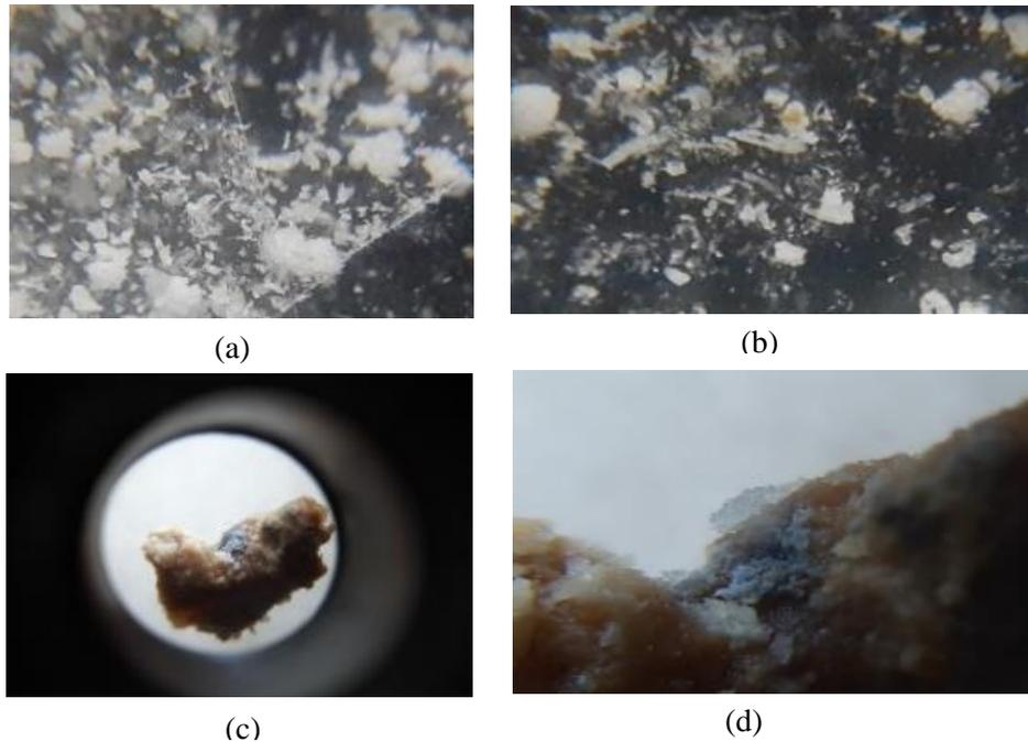
Figure 32 (a) and (b) mold sample collected from a lime plaster wall from different spaces. (c) and (d) mold sample collected from gap between wall and wooden door frame
