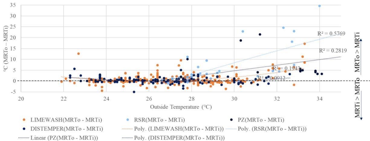
Figure 24 MRT performance for different categories of lime plaster survey cases.
