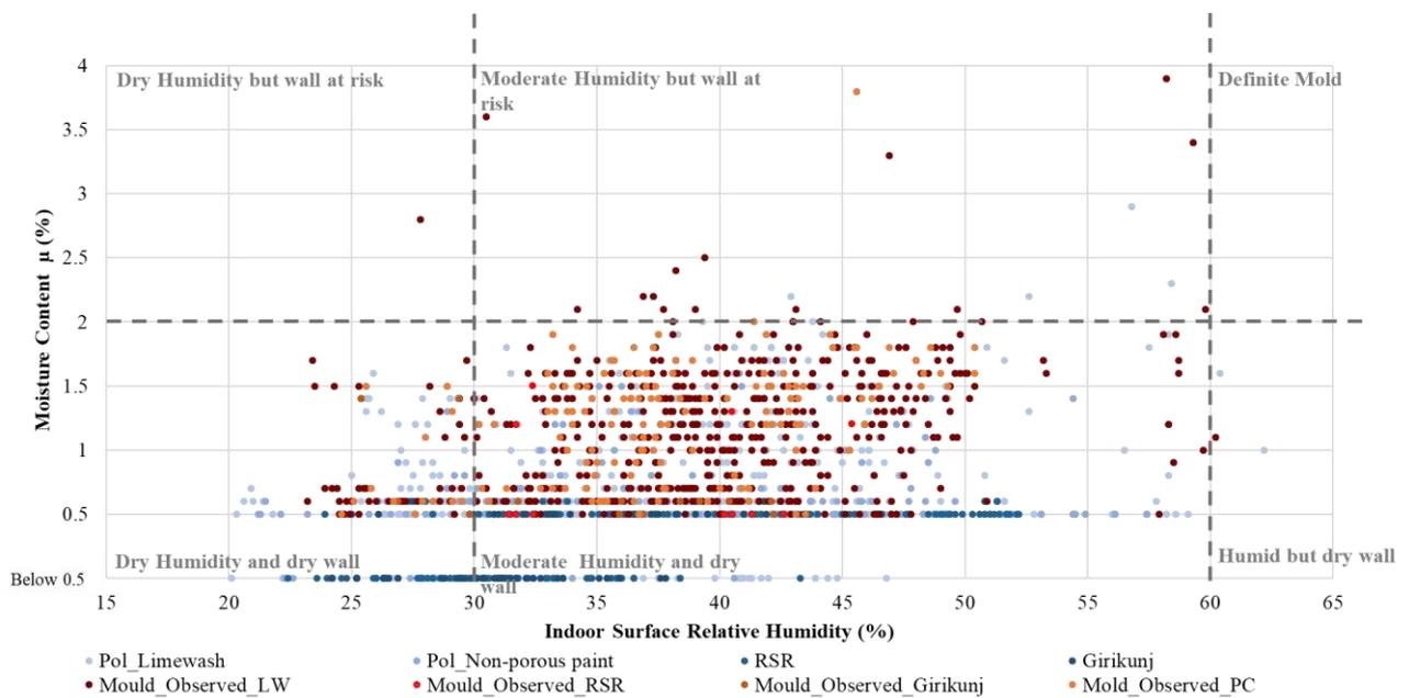
Figure 29 Moisture content Vs Surface relative humidity
