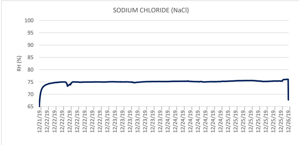
Figure 52 75% RH maintained by NaCl
