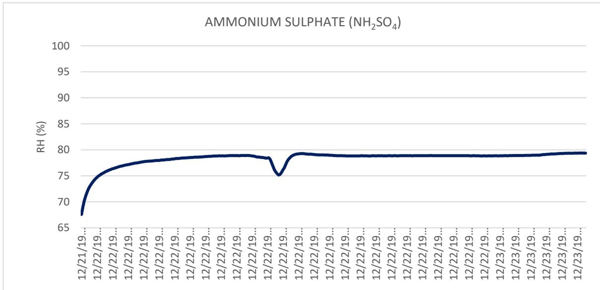
Figure 53 80% RH maintained by NH<sub>2</sub>SO<sub>4</sub>
