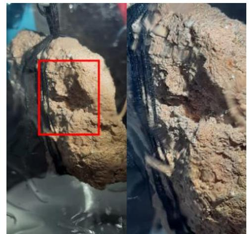
Figure 33 Mold growth on sample under 96% RH
