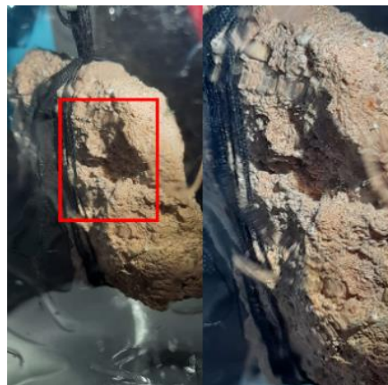
Figure 22 Mold growth observed under 96% relative humidity
