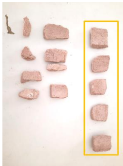
Figure 7 Lime plaster samples used for experiment Figure 6 Jars containing different salt solutions
