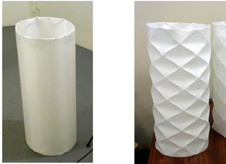
Figure 10. Prototypes of cylindrical 3D-PMA without surface unevenness (left) and with surface unevenness by means of the paper folding technique (right).
