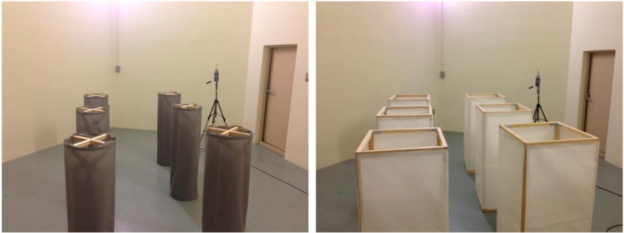
Figure 8. Prototype of 3D-PMA (left: cylindrical; right: rectangular) used in the experiment.
